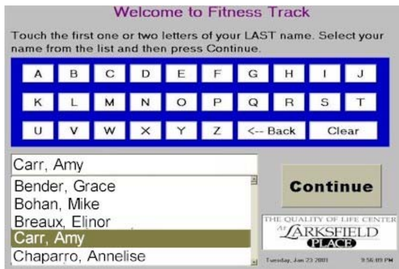
Figure 4. Revised FitnessTrack sign-in screen. Button sizes and font sizes were increased to insure more accurate touching.
